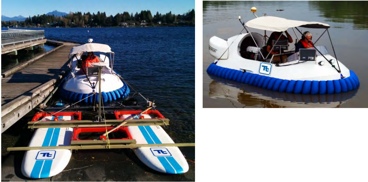
Figure 3-7. TtEC’s Hovercraft Survey Vessel
